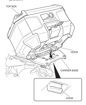
5. Secure the hook by push the release lever as shown.
