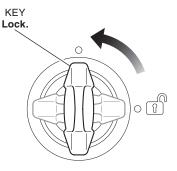
Remove the key. Be sure that release lever cannot be released.
