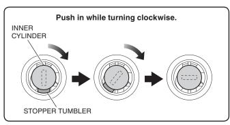
21. Draw out the key and check that the inner cylinder does not come out.
