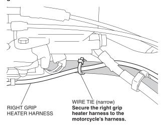
64. Secure the right grip heater harness with the wire tie as shown.
