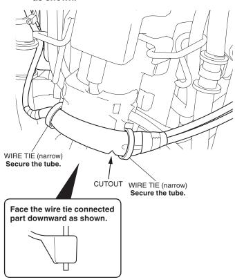
59. Secure the grip heater harness with the wire tie as shown.
