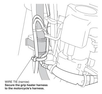
60. Secure the grip heater harness and left grip heater harness with the wire tie as shown.
