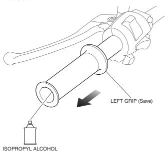
22. Using a isopropyl alcohol, remove all traces of adhesive from the left handlebar.
