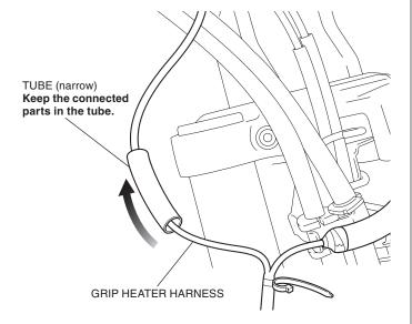
53. Secure the tube with electrical tapes as shown.
