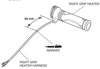
13. Install the clip band on the marked position as shown.
