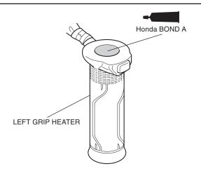
34. Apply Honda Bond A to the left handlebar as shown.
