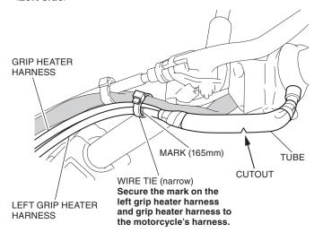
62. Secure the grip heater harness and left grip heater harness with the clamp as shown.
