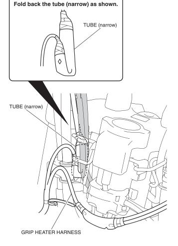
56. Secure the grip heater harness with the wire tie as shown.
