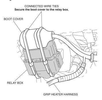
48. Secure the grip heater harness with the wire tie as shown.
