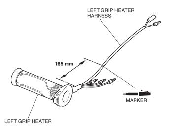
24. Cut the area of the tube as shown.
