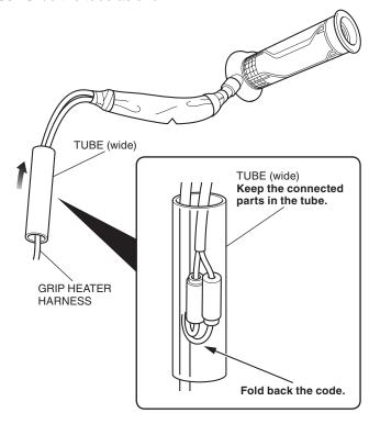
31. Secure the tube with electrical tapes as shown.
