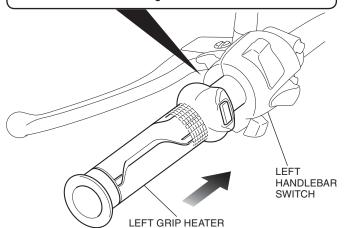
37. Pass the harness boot through the grip heater harness as shown.
