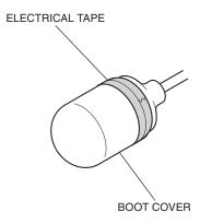
42. Cut the connector cover as shown.
