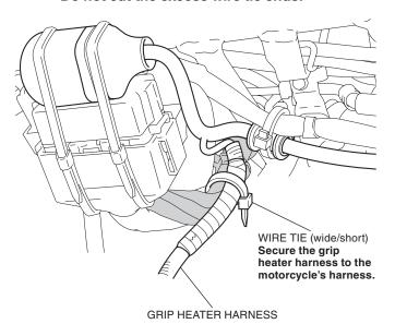
50. Pass the tube through the grip heater harness as shown.
