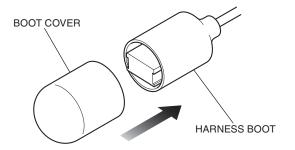
41. Secure the boot cover with electrical tape as shown.
