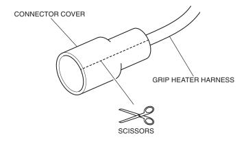
43. Remove the connector cover as shown.
