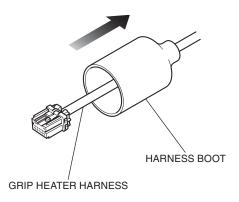
38. Connect the controller as shown.
