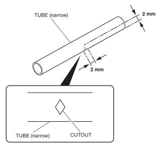
25. Pass the tube and cut tube over the grip heater harness as shown.
