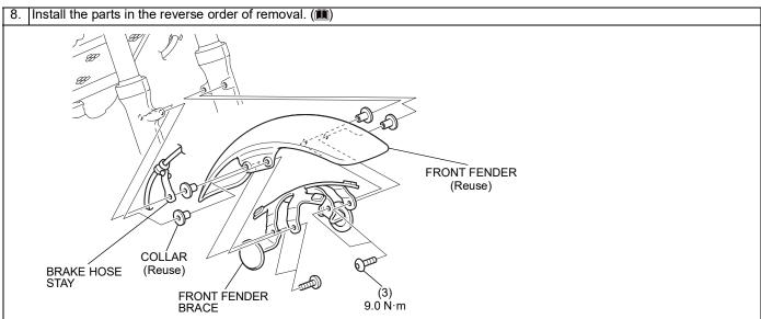
9. Install the motorcycle's parts in the reverse order of removal. (📵)
