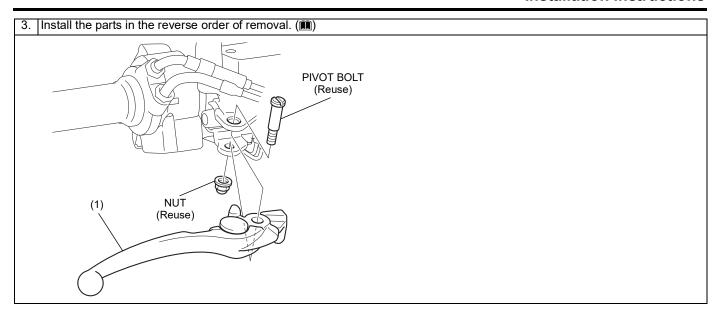
4. Check the lever for proper operation.
