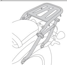
Remove the parts as shown. 1. Repeat on the right side. • <Left side> Motorcycle equipped with the Saddlebag support Ð 9 Т Ð 9 COÙLAR 0 WASHER LEFT SADDLEBAG SUPPORT PIPE BÒLT BOLT (Save) (Save)
